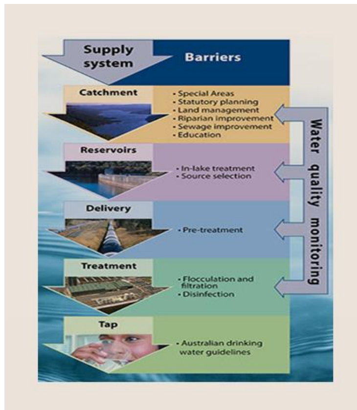
Fig. 5. The multibarrier approach traditionally used for drinking water treatment (Water NSW, 2021)
