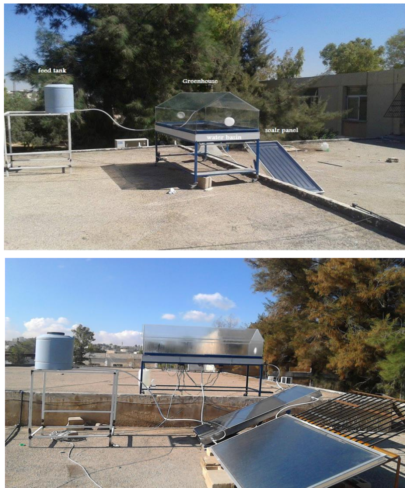
Fig. 1. Design of the solar still with – (a) Single solar panel; (b) Modified solar panel in series for accelerated evaporation during winter.
